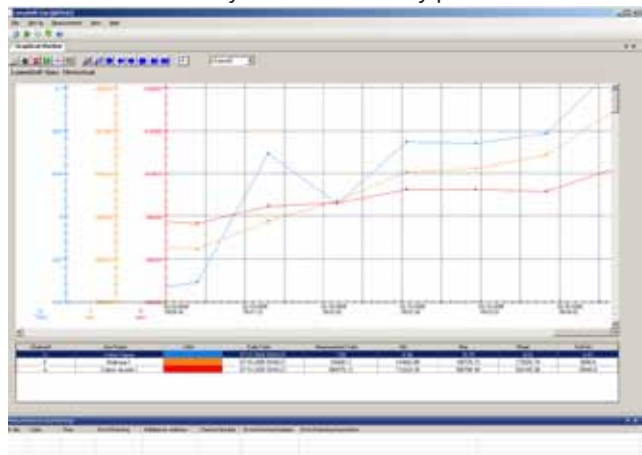
Fig. 1 The graphical window shows up to seven graphs. The user selects the data plotted, the scaling, the style and the color of the lines and the background to build the graphical window
