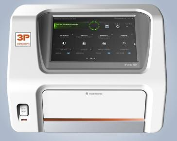
The density analysis of Powders, Foams and bulk solids
